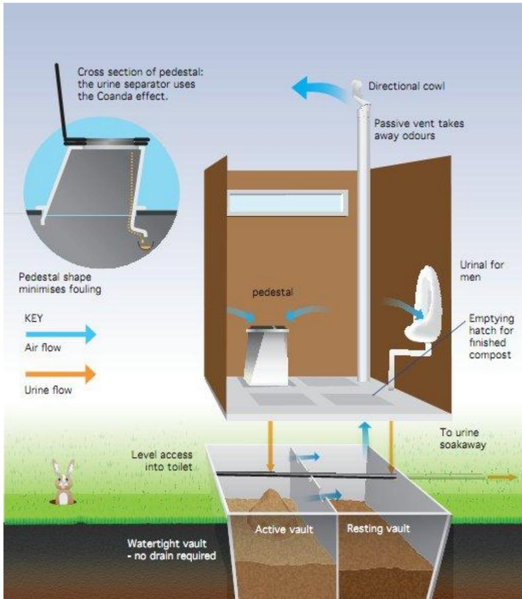
The toilet has two vaults used alternately for a period of not less than one year each. When the first vault is full, the second one is used. When that is full the first one is emptied of compost and brought back into use. Emptying takes place through the floor hatches.
